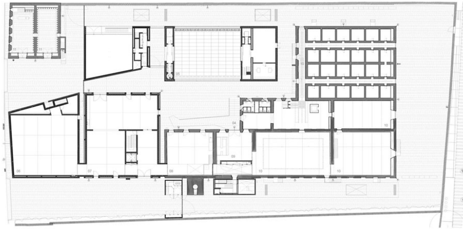
ARQUIPELAGO - CONTEMPORARY ARTS CENTRE GROUND FLOOR 04 - Foyer 05 - Auditorium and multipurpose area 06 - Storage area 07 - Workshop and carpentry 08 - Assembly and disassembly of exhibitors 09 - Entrance hall and reception 10 - Exhibition area 11 - Museum shop and bookstore 12 -
